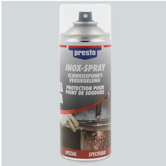
presto Inox-Spray is a reliable corrosion protection as well as a surface coating. Seals weld spots and weld seams. Also applicable as corrosion protection during spot-welding between car body sheets.
